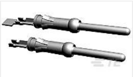
TE 产品编号1-66359-2 III+ PIN,18-14,30AU/FL,STRIP
