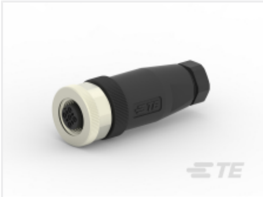
TE 产品编号T4110001041-000 M12,FEMALE,STRAIGHT,A CODE,4P,PG7,GOLD
