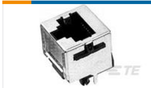
TE 产品编号2-1734858-3 RJ11,8P8C, TOP ENTRY, SMT, 30u"
