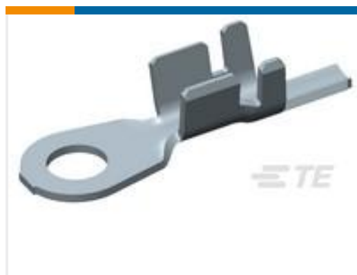
TE 产品编号881016-2 RING TONGUE 6.0-10.0 MM2 1.00X22.7 TPBR
