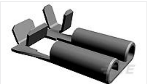
TE 产品编号1742089-2 187 FASTON,FLAG,REC.,18-14OR2X18AWG,TPBR
