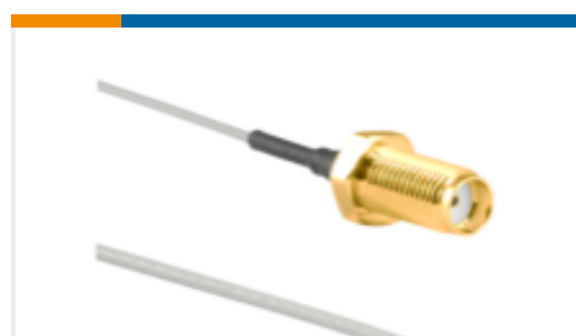
TE 产品编号CSI-SGFB-200-UFFR SMA to U.FL/MHF1 200mm 1.13 OD
