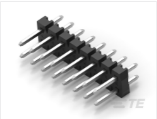
TE 产品编号 1-2842126-0 20P,2MM,BRK HDR,DRV,T,2.8,0.1AU,TB
