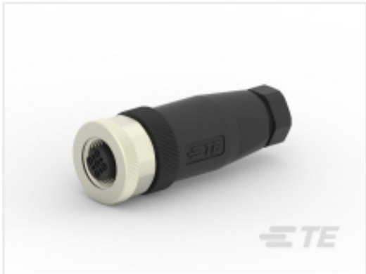
TE 产品编号T4110401051-000 M12,FEMALE,STRAIGHT,B CODE,5P, PG7,GOLD
