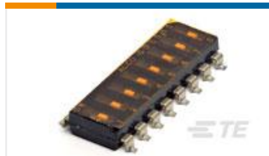
TE 产品编号1-1825006-9 GDS10S04=DIP SW,SLIDE,SMT
