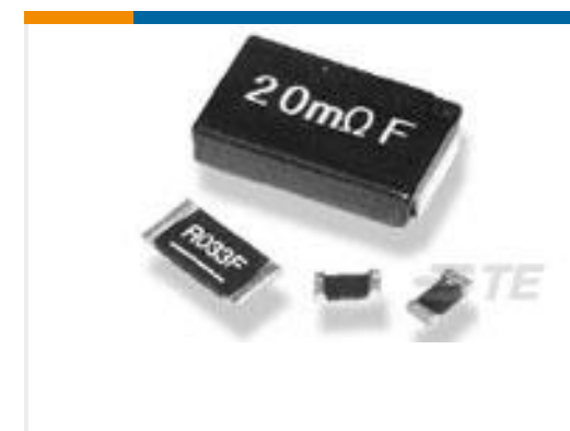
TE 产品编号2176157-8 TLM 2010 0.75W R039 5% 100PPM 4K RL
