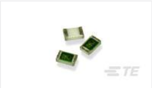
TE 产品编号 1614902-3 CPF0805 1K5 0.1% 25PPM 5K RL
