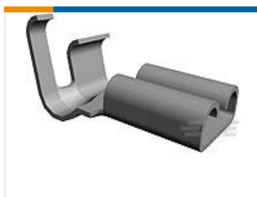
TE 产品编号1742370-2 187 FASTON,FLAG,REC.,18-14 AWG, TPBR
