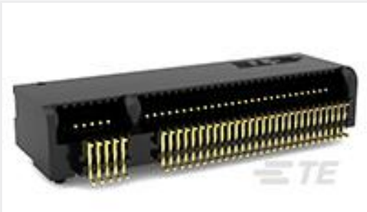
TE 产品编号2199230-7 M.2 0.5PITCH 4.2H KEY A GOLDFLASH
