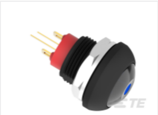
TE 产品编号2329387-5 PB OFF/ON FC BLK M1 TERM BLU LED IP68
