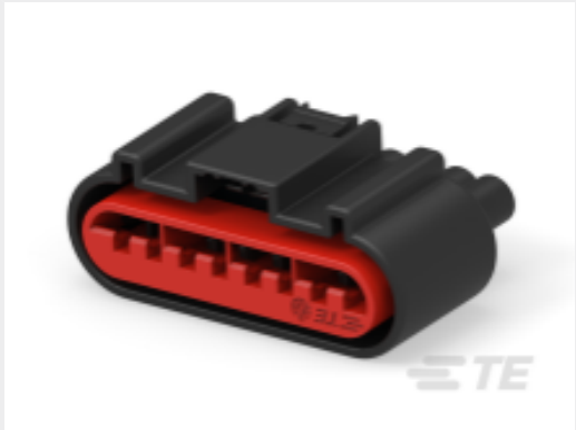
TE 产品编号2112058-4 8POS,YES 1.5,SOCK HSG,ASSY, SEALED
