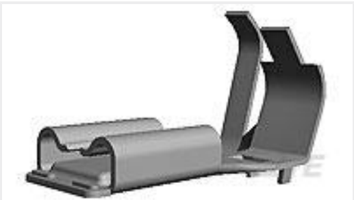
TE 产品编号175193-1 187 PL EX FLAG REC. 22-16AWG TPBR
