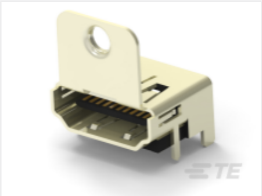
TE 产品编号 1-1747981-4 Std HDMI, RA, SMT, Panel grd, Flange
