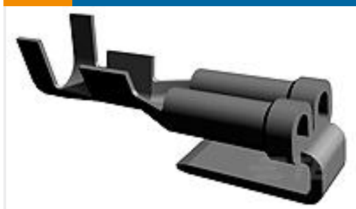
TE 产品编号62003-2 110 FASTON REC 22-18 AWG TPBR
