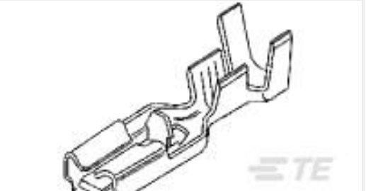
TE 产品编号63809-1 PL 250 TERMINAL REC 18-14 AWG TPBR
