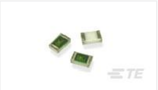
TE 产品编号5-2176091-7 RP 2A 0.25W 226R 0.1% 25PPM 1K RL
