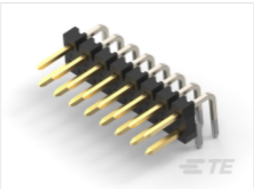
TE 产品编号1-2842162-0 20P,2MM,BRK HDR,DRRT,2,8,0.1AU, BOX
