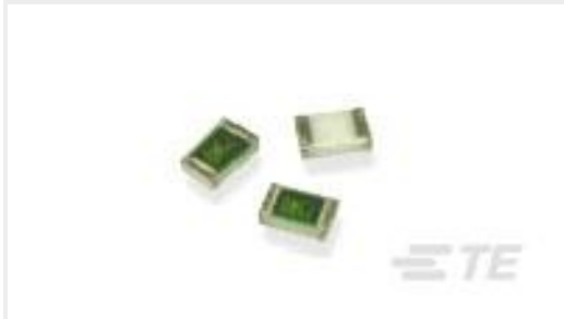
TE 产品编号1-1614352-3 RN 0603 22K1 0.1% 10PPM CUT LENGTH
