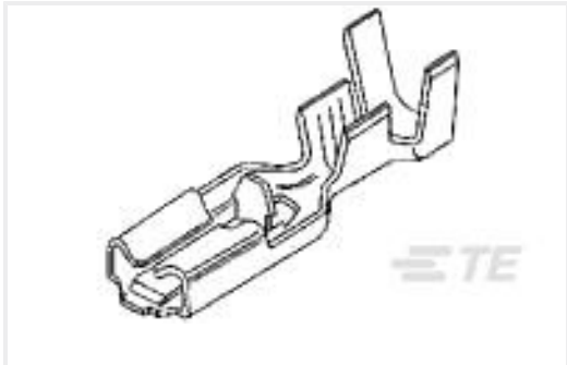
TE 产品编号173690-1 PL 187 TERMINAL 24-20 AWG 0.3 X 14.0
