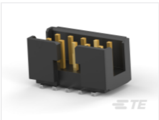
TE 产品编号1-2373376-0 10P,2MM,SHRD HDR,DRV,T,SMD,0.1 AU,TB
