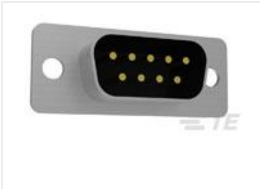
TE 产品编号5-747904-2 9 Plug Solder Cup, Gold Flash,
