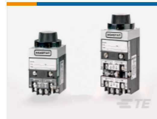
TE 产品编号 1-1472969-5 7022RCA2T=RLY,STD,OFF,2P,60VDC, 15SEC,A2,
