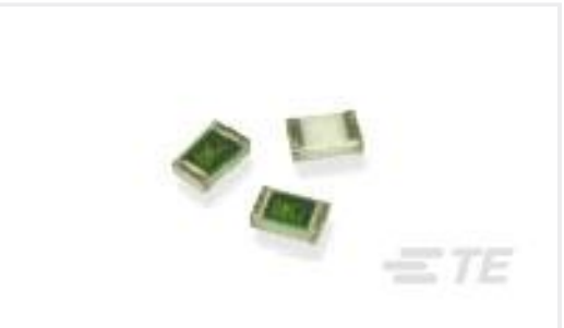
TE 产品编号5-2176092-0 RP 2A 0.25W 2K43 0.1% 25PPM 1K RL
