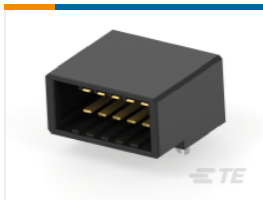
TE 产品编号178308-3 Header Assembly: Wire-to-Board, 15A, gold or tin plated
