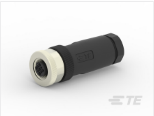
TE 产品编号T4110402021-000 M12,FEMALE,STRAIGHT,B CODE,2P, PG9,GOLD
