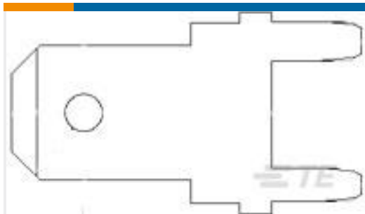
TE 产品编号1217057-1 187 FASTON,PCB TAB,TPBR
