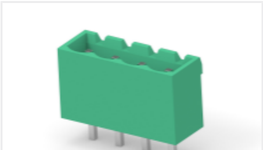
TE 产品编号2351885-4 4POS TB HDR 180 DEG, PITCH 5.0&TL 4.5mm
