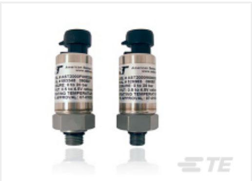
TE 产品编号11100520-00 448 BAR, 7/16-20UNF Male,0.5-4.5V ratiom
