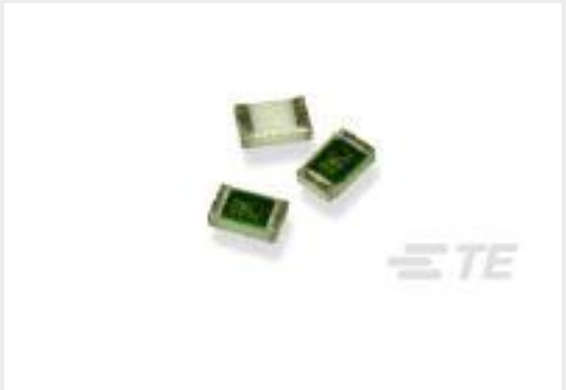
TE 产品编号3-1614890-0 CPF 0805 11R3 0.1% 25PPM 1K RL
