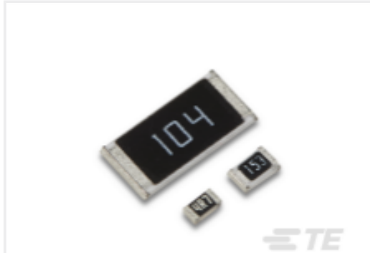
TE 产品编号1-2176343-4 CRGCQ 1206 120R 1%
