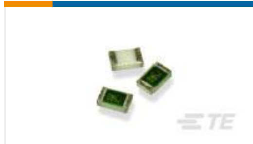
TE 产品编号7-1879208-6 CPF 0402 13K 0.1% 25PPM 1K RL
