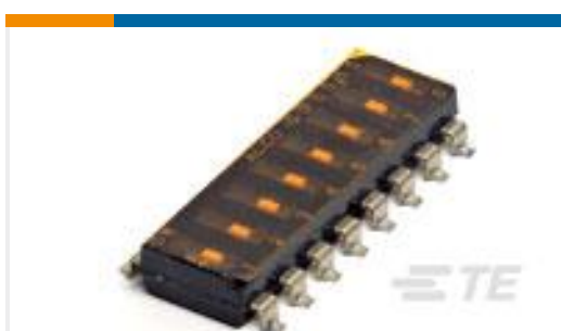
TE 产品编号1-1825006-9 GDS10S04=DIP SW,SLIDE,SMT
