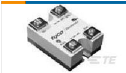
TE 产品编号1393030-7 SSR-240D25= PANEL MOUNT, 25A, 240VAC-DC i/p
