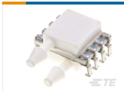
TE 产品编号4515DO-DS3BK004GP 4IN PCB MOUNT I2C PRESSURE SENSOR
