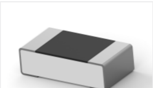
TE 产品编号2-2176372-2 RQ 0603 82K5 0.1% 10PPM 5K RL
