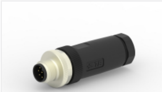
TE 产品编号T4111001081-000 M12,MALE,STRAIGHT,A CODE,8P, PG7,GOLD
