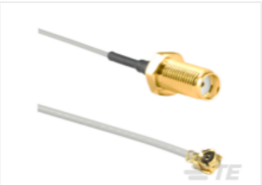
TE 产品编号CSI-SGFB-200-UFFR SMA to U.FL/MHF1 200mm 1.13 OD
