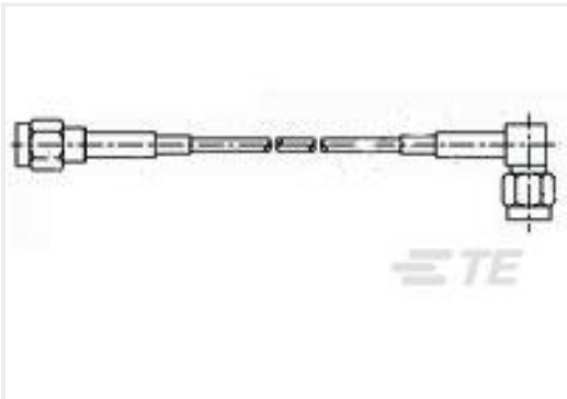
TE 产品编号1337810-1 50 OHM COAX SMA STR PLUG ELB P
