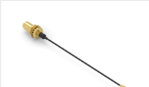
TE 产品编号2016682-2 RF CA,UMCC1 TO SMA JACK,1.13MM, L100MM
