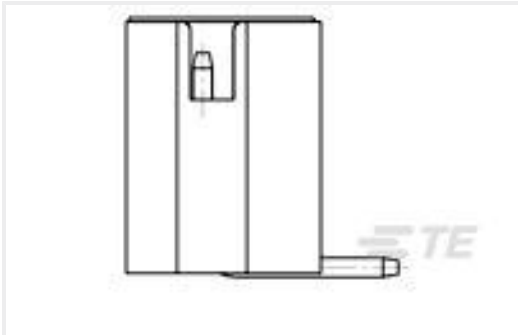
TE 产品编号1775470-4 HPI CONN., 2.0MM, V/T, SMT, 4P, 80U"
