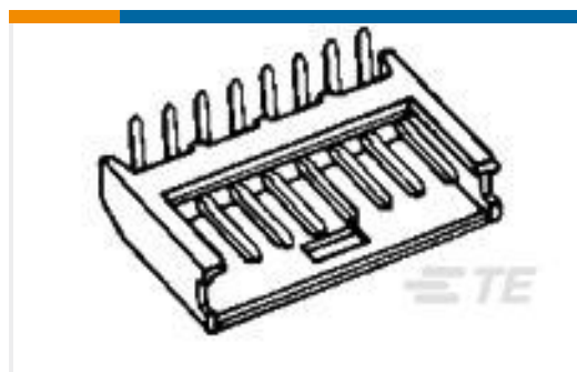
TE 产品编号280379-2 6P MODU II SHRD HDR, RT ANG, 0.38 AU
