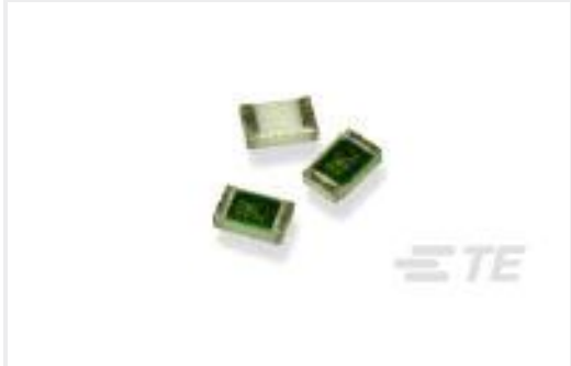
TE 产品编号9-1879208-6 CPF 0402 91K 0.1% 25PPM 1K RL
