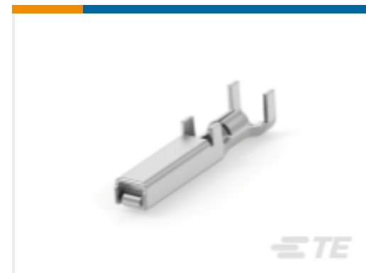
TE 产品编号1-353715-2 Contact: Component To Wire; 15A, 28-14 wire size
