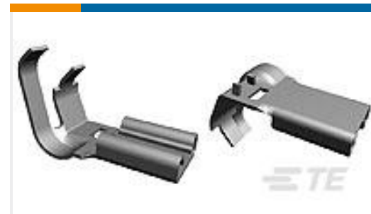
TE 产品编号42404-1 250 FASTON FLAG REC 18-12 AWG NPST
