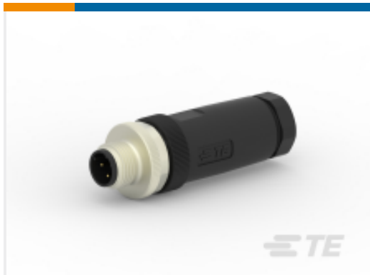
TE 产品编号T4111502041-000 M12,MALE,STRAIGHT,D CODE,4P, PG9,GOLD
