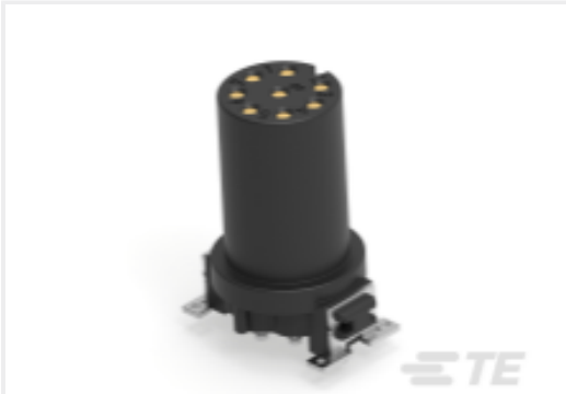
TE 产品编号494166-E M12 FEMALE, A CODE, 8P, 17MM SMT
