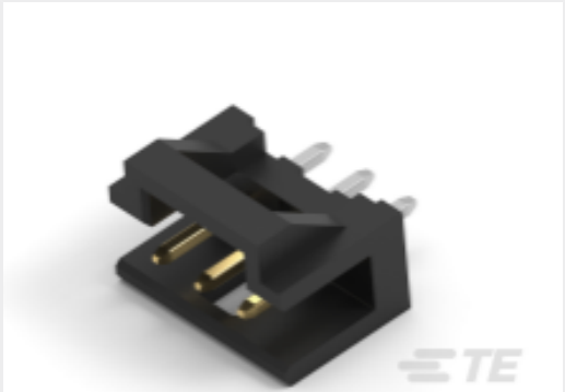
TE 产品编号2823402-4 4P,2MM,PL HDR,SRVT,2.8,0.76AU,TB
