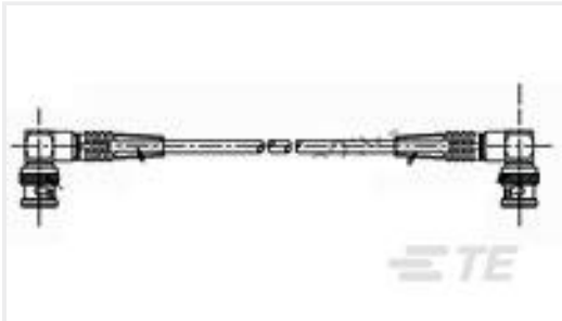
TE 产品编号1337773-4 50/OHM COAX BNC ELB PLUG ELB P
