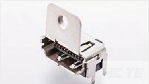
TE 产品编号1-1747981-1 Std HDMI, RA, SMT, Panel grd, Flange
